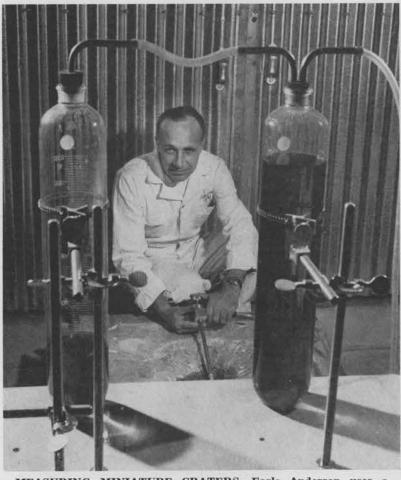
MEASURING MINIATURE CRATERS, Earle Anderson uses a separatory funnel apparatus to precisely measure the volume at various levels in both the "apparent" and "true" model craters.
